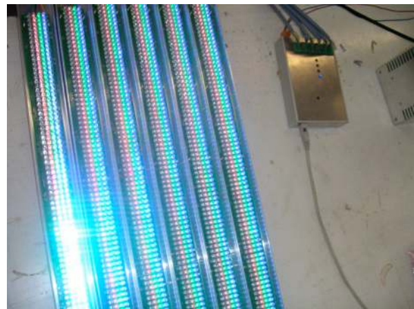
4-color LED-stripes, mounted in u-profiles
