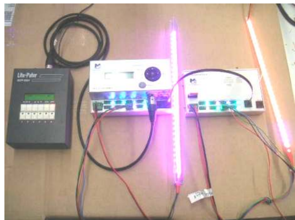
DMX-source, master, 8-channel slave and LED-teststrips
