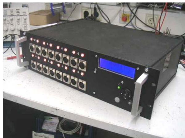
16-channel rack Meira1916 as prototype
