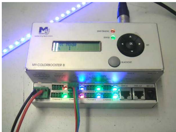
DIN-rail master My-Colorbooster8 with a LED-teststripe
