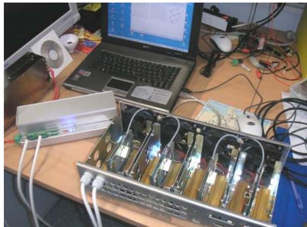
test environment with PC, power supply and dummy load
